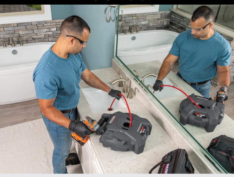
The NEW RIDGID<sup>®</sup> FlexShaft K9-12 machine is the most compact version of the FlexShaft Drain Cleaning Machines. The fully enclosed housing contains 30' of FlexShaft cable, encapsulated in nylon sheath for less mess and easy cleanup. The lightweight, portable design is perfect for  $1^{1}/_{4}$ " - 2" pipes.
