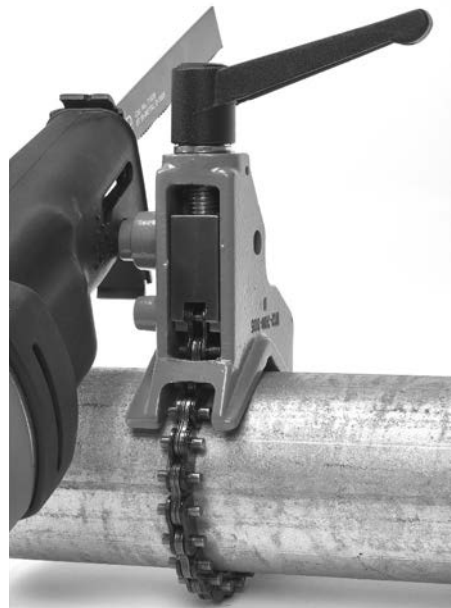
Figure 13 – Mounting Saw on Support Device
