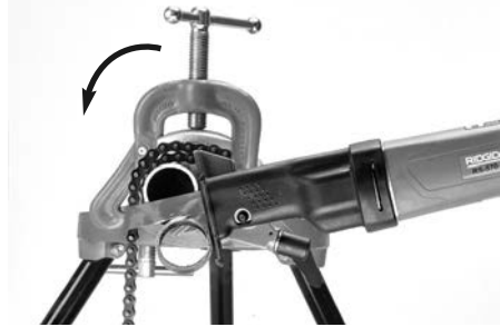
Figure 15C– Cutting the Pipe
